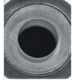
Kel-F valve seats of line valves in HBr Service, with NANOCHEM® purifier, 1000 cycles.
