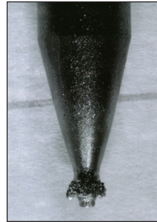
Without Purification Tungsten Deposits on electrode (5/32", EWTh-2)
