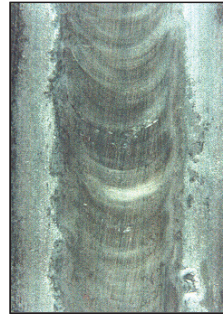
Without Purification (Impurity Content = 40 ppm) Surface Oxides, Porosity, Poor Cleaning Action, Poor Wetting Rough Weld Surface
