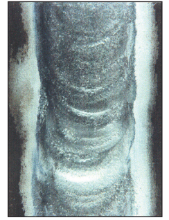
With Purification No Porosity, Clean X-Rays Good Cleaning Action, Excellent Wetting, Excellent Ductility Very Smooth Surface
