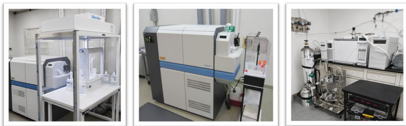
Figure 4: Application of state-of-the-art analytical techniques capable of detecting contaminants at ppt and ppb levels to support product development, quality assurance, and contamination investigations.
